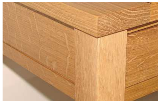
▲ Pic.2 To add interest, the side rails were detailed with a 3mm groove that continues the line of the drawer opening
